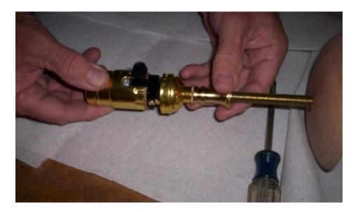
Press the bulb socket firmly into socket base.
