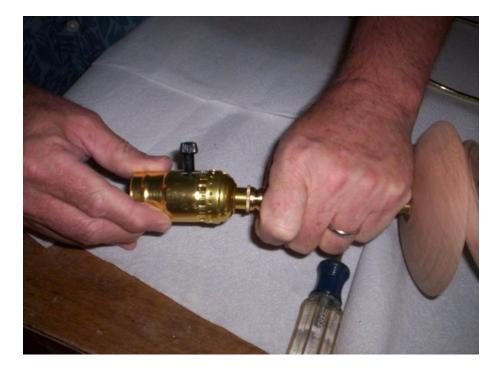
14. Fit the socket cover over the bulb socket and press firmly into the socket base. Use firm pressure...it will lock evenly into place and you should NOT be able to pull it back out.
