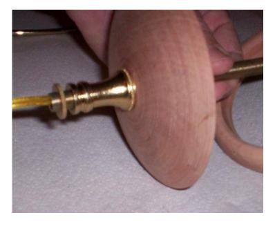
8. If not using the harp, slide the ferruled lock nut down to the brass neck.
