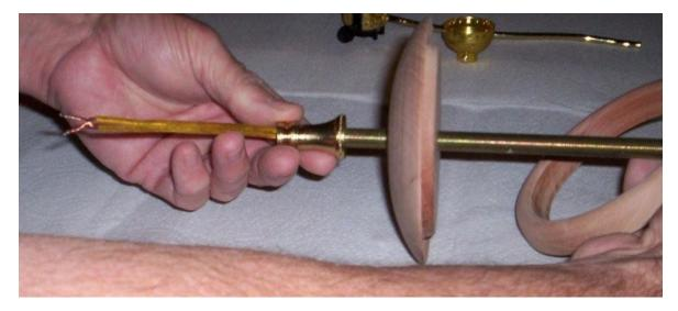
5. Slide threaded brass neck down snugly to the lid. Do NOT over tighten at this point, as this will deform the basket.
