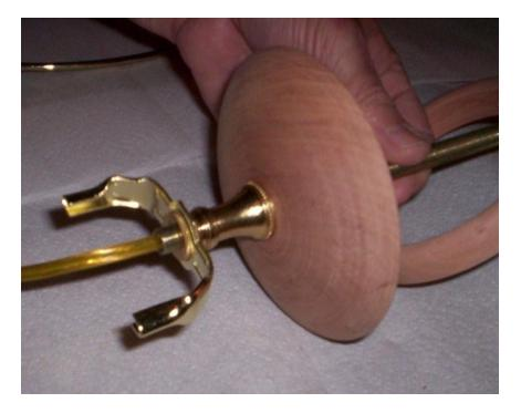
7. If you are using a harp, install the harp base now. Lock it in place with ferruled lock nut.
