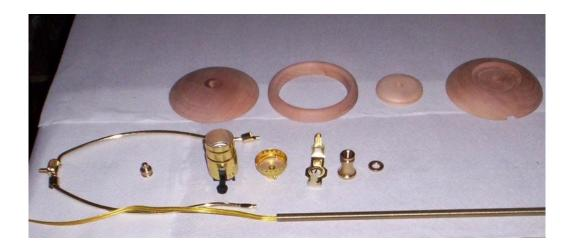
2. The parts laid out in order. Dry fit everything together and measure rod to length. Screw small nut onto rod and cut off rod with hack saw.
