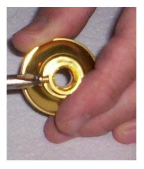
Loosen set screen in threaded socket base.
